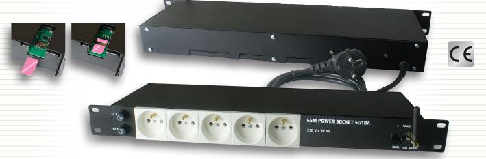
Power strip in Rack 19" standard equipped with 5 independently managed 230V sockets and GSM module for sockets remote control. Managing sockets can be performed via SMS messages with authentication password. Power GSM module is supported by the battery, so that the proper programming can be notified of the lack of power and return.
