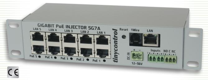
**Gigabit PoE injector** is manufactured in our company to the needs of operators, wireless internet. As the only passive PoE device can deliver up to 1.5A power supply cable Ethernet standard 1 Gb/s. This effect was achieved using special, high current transformers on signal lines ethernet manufactured in Poland for our order. Power signal is introduced only four lines in accordance with the passive PoE 100 Mb/s, so that the device is completely compatible with the slower version of the LAN.
