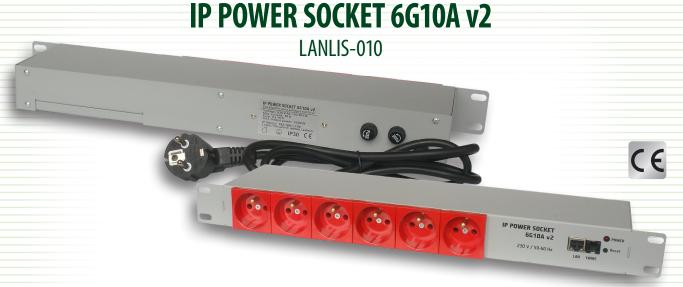
Power distribution unit in Rack 19" standard. Equipped with six independly managed outlets for 230V. Managment available by embeded web server or SNMP protocol. Except ethernet socket ther is 1wire socket for temperature measurement. In addition to the Ethernet port, the unit has an input for temperature sensors as standard 1wire (DS18B20). It is possible to support up to 4 sensors (on sale splitter 4 to 1).
