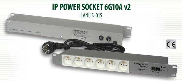
Power distribution unit in Rack 19" standard. Equipped with six independly managed outlets for 230V. Managment available by embeded web server or SNMP protocol. Except ethernet socket ther is 1wire socket for temperature measurement. In addition to the Ethernet port, the unit has an input for temperature sensors as standard 1wire (DS18B20). It is possible to support up to 4 sensors (on sale splitter 4 to 1).
